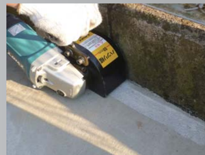
Works on concrete surfaces at the edges, and hard to reach areas.
