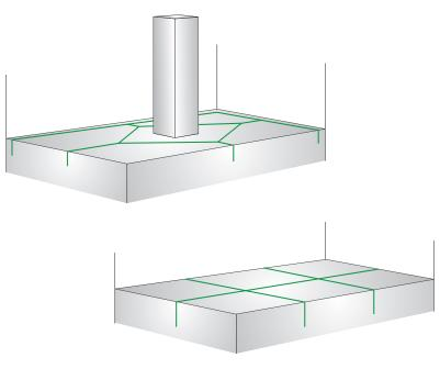
A key reason to cut grooves is for the installation of heavy-duty polyurethane flooring systems, to strengthen the bondage of materials to the substrate.
